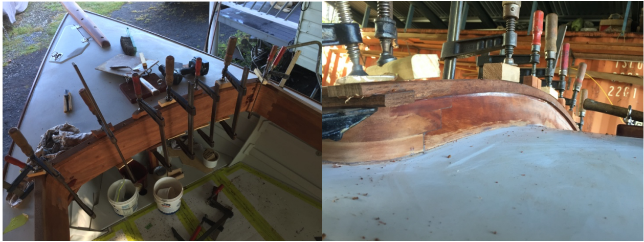
The last coaming grab rail has now been permanently fitted. Trimming & sanding, then varnish & done!
